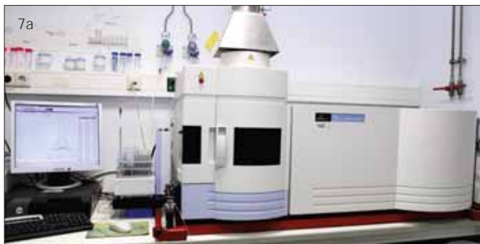
Fig. 7a and 7b ICP spectrometer used for analysis of the metal ions released into the solution and determination of the loss of mass
